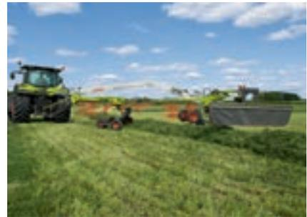
Up to 27.5 in (70 cm) lifting height for ease of turning at headlands
