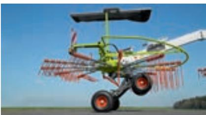
Generous lifting height for driving over windrows at headlands: up to 23.5 in (60 cm) in the LINER 700 TWIN
