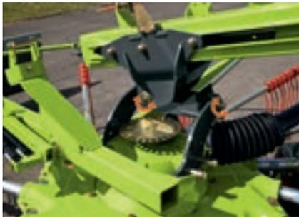
Fully floating rotor suspension
