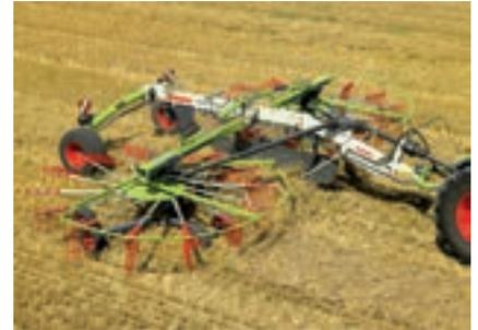
Central rakes like the LINER 2900 are very suitable for use in straw.
