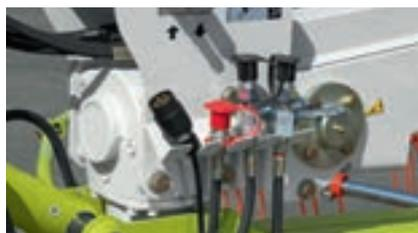
Hydraulic sequential control fitted as standard to adjust the time delay between front and rear rotors when raising and lowering
