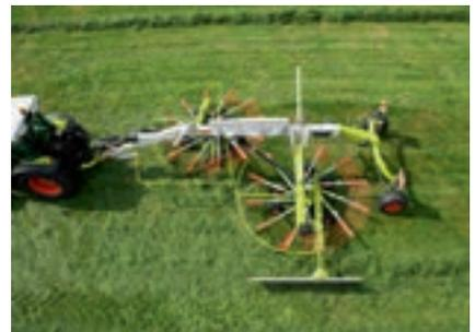
Tidy forage transfer from the first to the second rotor
