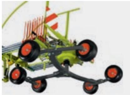
Six-wheel chassis: with extra tandem axles and trailing wheels for precise ground-contour tracking
