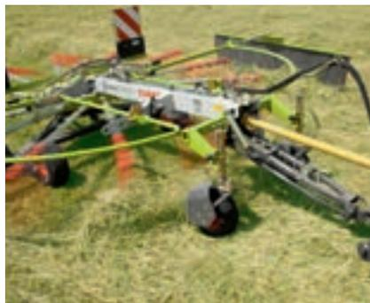
In virtually all of the single-rotor rakes, the guide wheel is available as an optional extra
