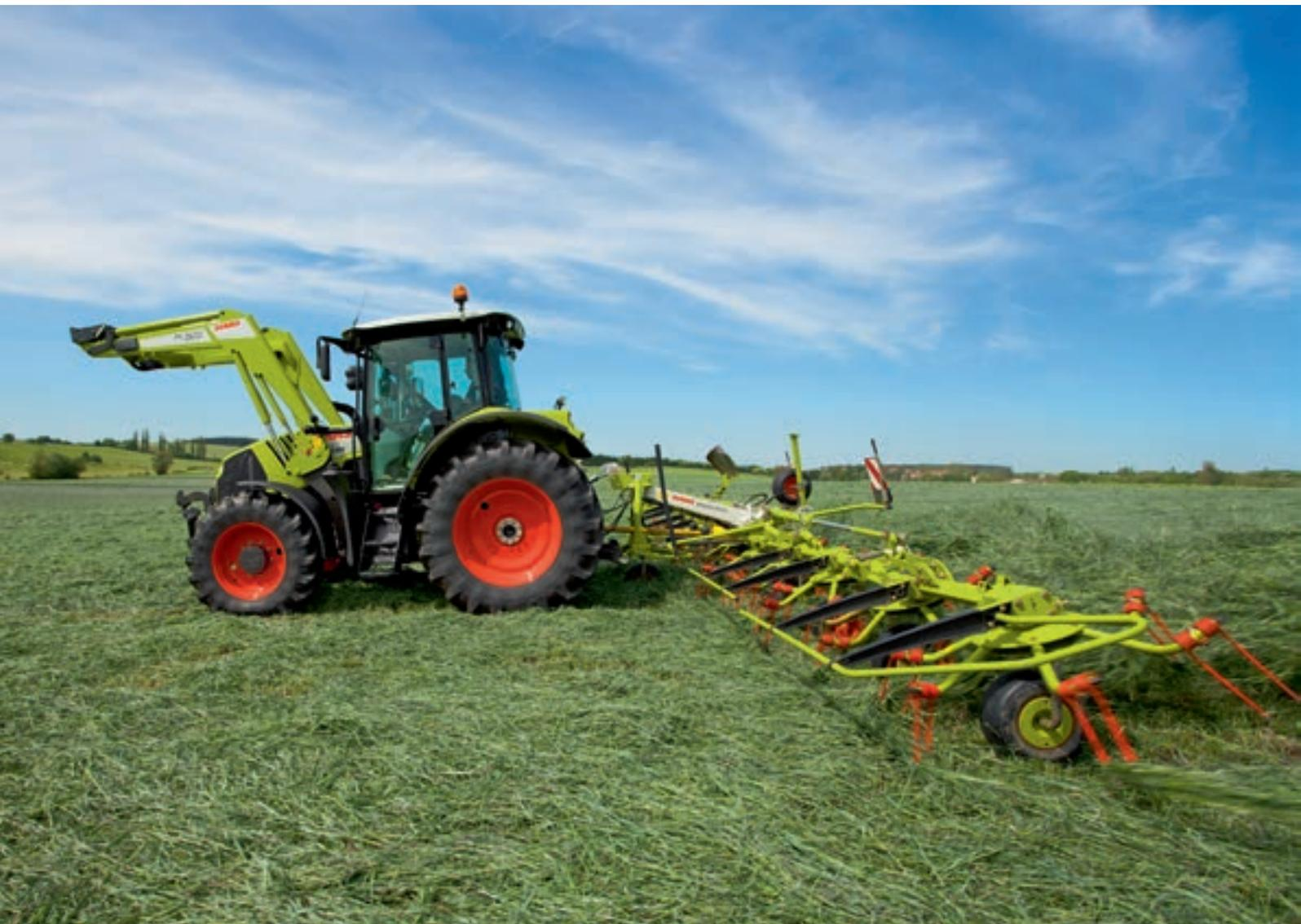
Ten rotors for three-point linkage attachment.
